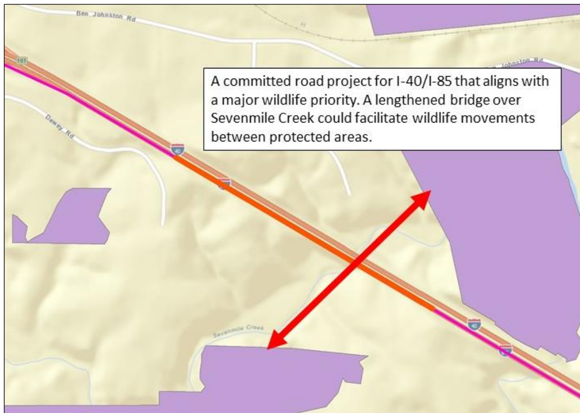
Figure 12. A committed road project on I-40/I-85 for the draft 2018-2027 STIP (pink) aligns with a major road priority in our All-Species model (orange). This road segment scored a 7 due to high traffic volume (for both large and small species), road width, impermeable median, high speed, importance for box turtle centrality, and the presence of a Natural Heritage Element Occurrence. Overlaying this data allows conservation groups to better comment and provide recommendations to NCDOT on how to include appropriate wildlife mitigation into road project design. For example, lengthening a bridge over Sevenmile Creek so that there is terrestrial passage on either side of the waterway would help to facilitate wildlife movement between an Orange County easement to the northeast and Sevenmile Creek Park to the southwest (red arrow).
